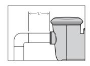
\*NOTE: It is recommended that a minimum length of straight piping (shown as "L" in diagram to the right), equivalent to 5 pipe size diameters, be used between the pump suction inlet and any plumbing fittings (elbows, valves, ect).
